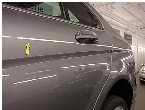
9. Tür hinten links Delle/ Kratzer smartrepair
